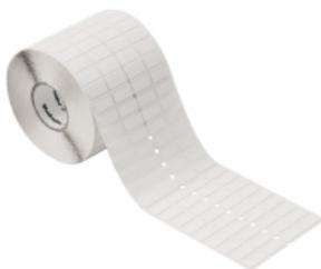
THM GEW woven-fabric labels are made from a very flexible cotton fabric. Delivery on reels for use with thermal transfer printers enables an adhesive layer which is thicker than that of A4 sheets for office laser printers. Together, this flexibility and the thick adhesive layer ensure higher adhesive strength and enable use on angular or round objects such as e.g. cables or hoses.
